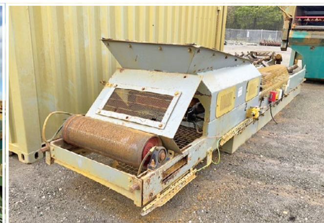
34M CONVEYOR BELT
