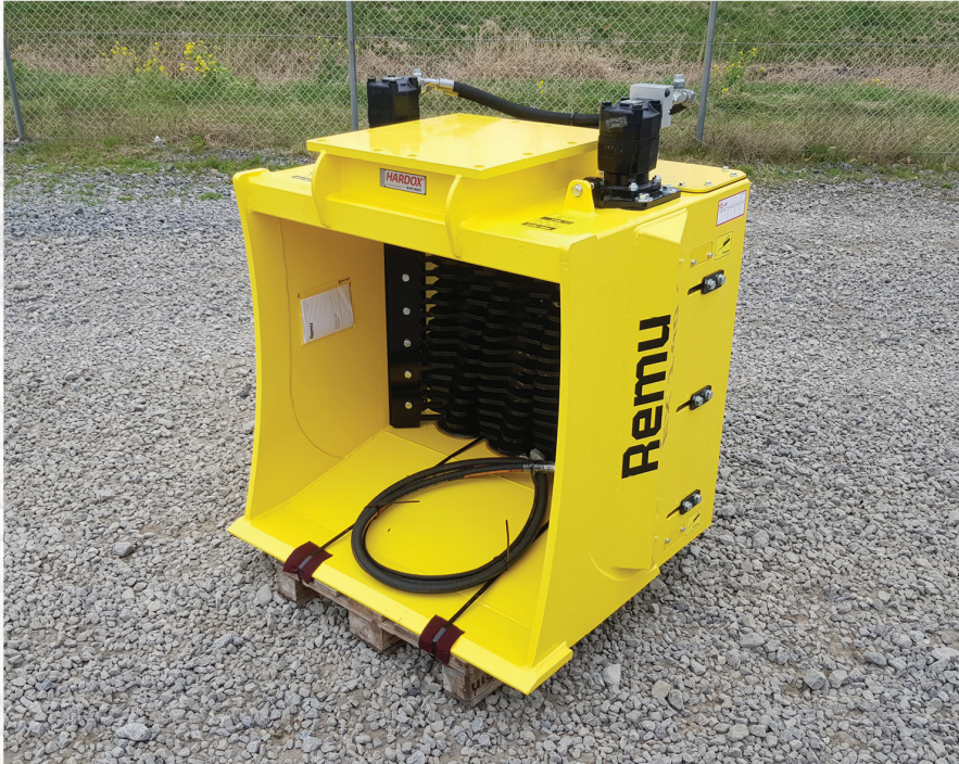
REMU EX140 | 2022 screening bucket 16t or heavier excavators bucket volume 0,9 m3 (ISO) weight 1400 kg screening blade with 34mm blade spacing
