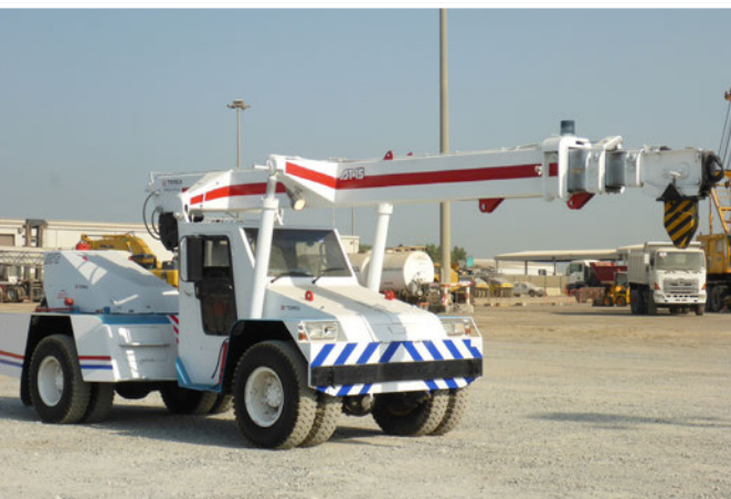
TEREX FRANNA AT15 15 TON HYDRAULIC MOBILE CRANE
