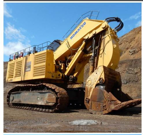
Year 2012 Manufacturer Komatsu Model PC5500-6E Asset Type front shovel Serial Number 15122 Usage TBD Comes with (2) ABB, electric, 900 kw, 14 ft bkt, 3 view camera, fire sup system
